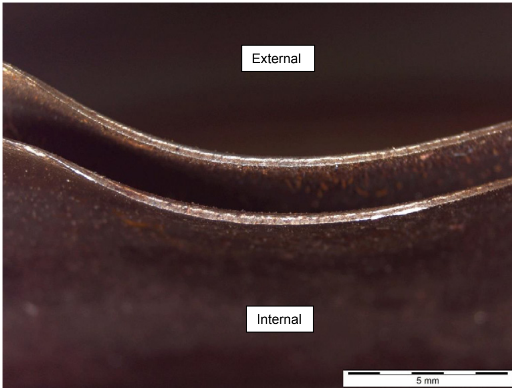
Figure 7. Detail of the fracture surfaces along the circumference, some plastic deformation appeared to be visible.
