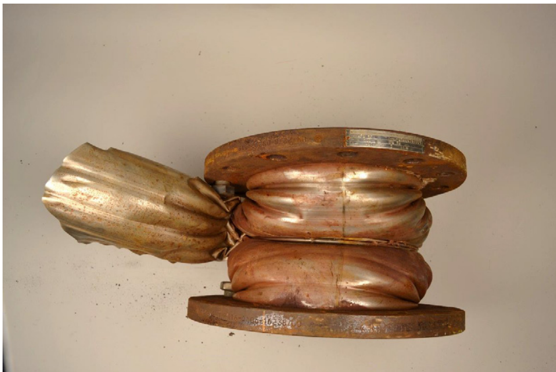
Figure 3. The unfractured side of the bellows with expanded convolutions adjacent to the central compressed convolutions. The central convolutions are obscured by the expanded convolutions on each side.
