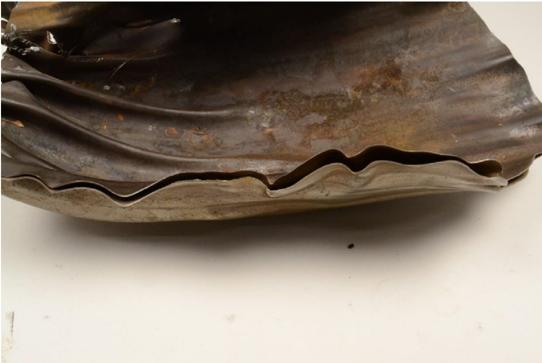
Figure 5. The fracture across along the side or circumference of the bellows illustrating the exact same fracture path through both bellows plates.
