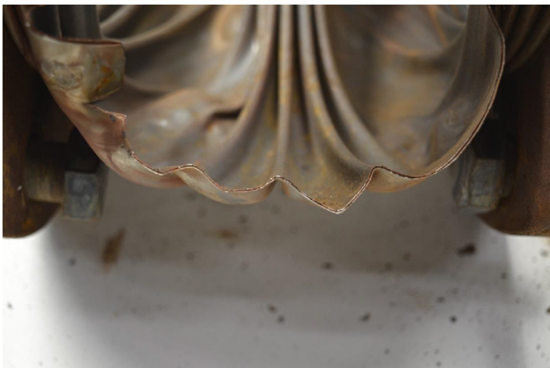
Figure 4. The fracture across the width of the bellows illustrating the exact same fracture path through both bellows plates.
