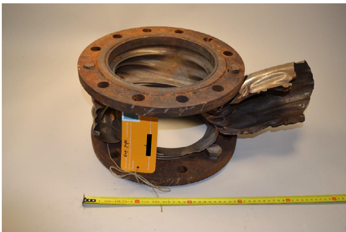
Figure 1. The failed expansion joint as received by Element Materials Technology, Amsterdam.
