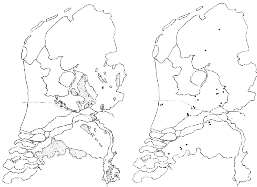
Figure 5.2-2. Maps showing the distribution of rattle stones in the Dutch pre-Saalian Pleistocene (left) and presence of siderite concretions at a depth of more than 20m in boreholes in fluvial pre-Saalian Pleistocene deposits (right). Dotted line: ice-frontline of the Saalian glaciers at their widest extension; stippled areas: outcrops of the fluvial pre-Saalian Pleistocene (derived from Van der Burg, 1970).
