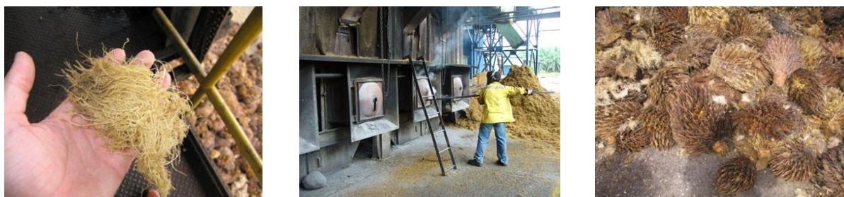
Figure 3.1.2.1. Picture of mesocarp fibre that is used as fuel for generating steam at the mill and of EFB (empty fruit bunch)
