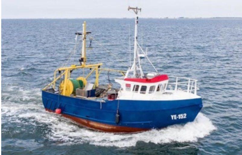
Figure 2.14 – YE 152 'Meru' (formerly SCH 87) with MMSI number 244727000. Equipment on the lower (stern) deck was adjusted to equipment specific for the type of fishing: gillnets or pots. This vessel was used for multi-species pots and gillnet fishing.
