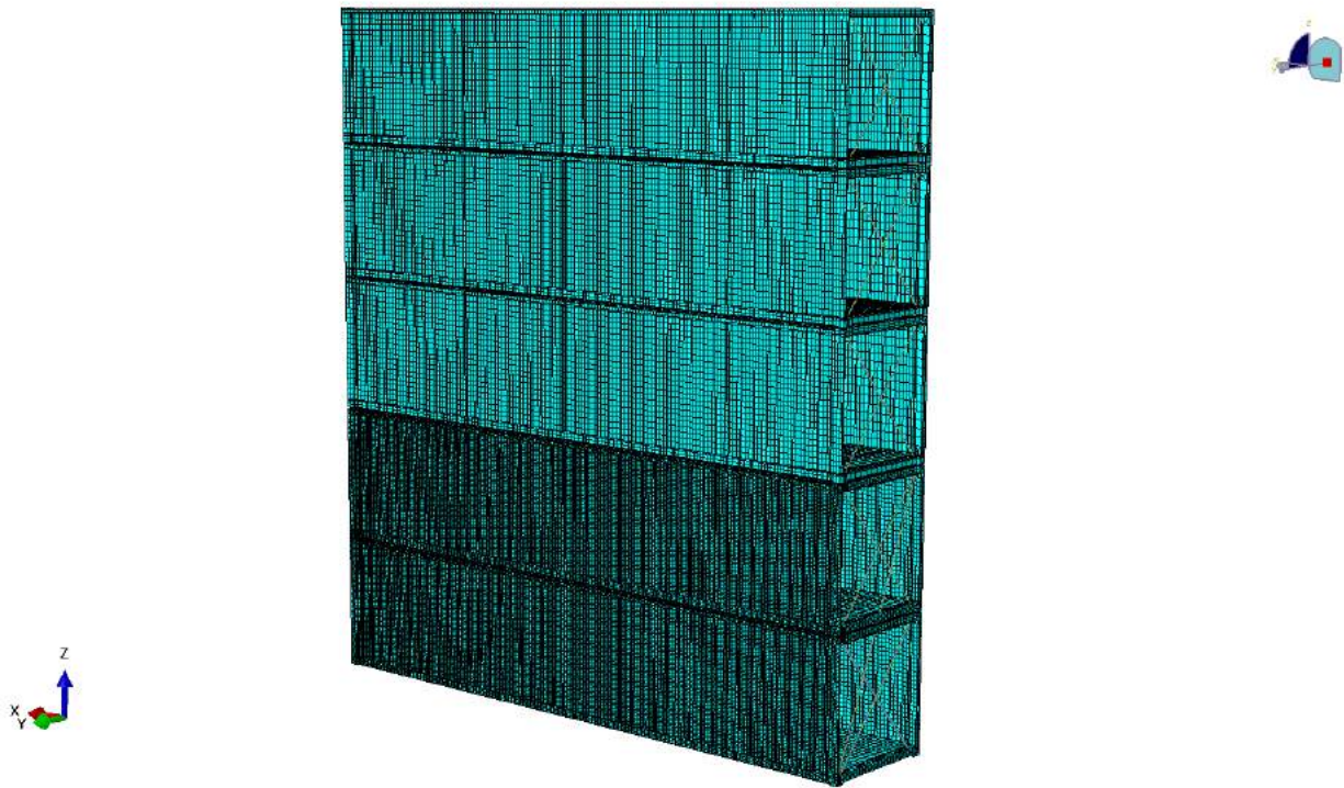
Figure 5-2: FEM mesh of the container stack
