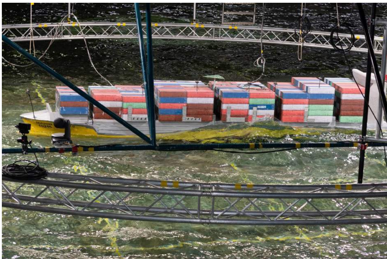
Photo 14 Test 33327_01OB_04_004_009_01: \mu = 270^\circ – H_s = 4.5 m – T_p = 8.5 s
