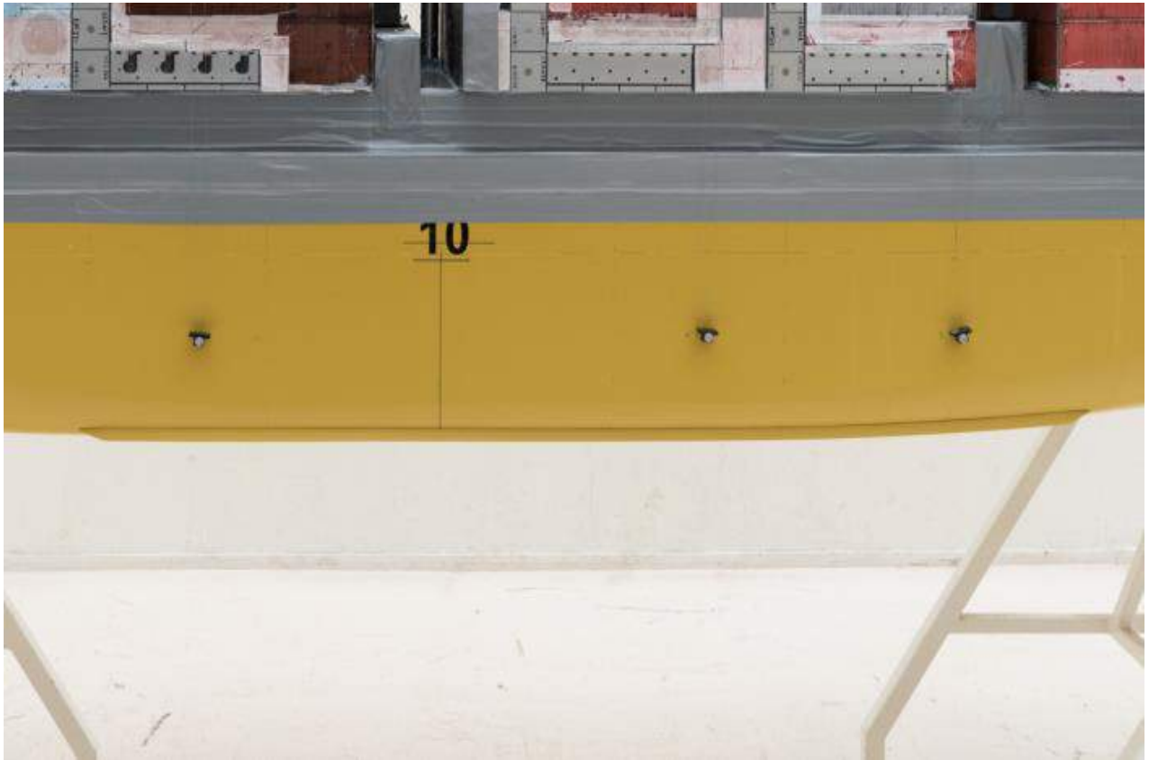
Photo 8 Details of the bilge keels – LC 2
