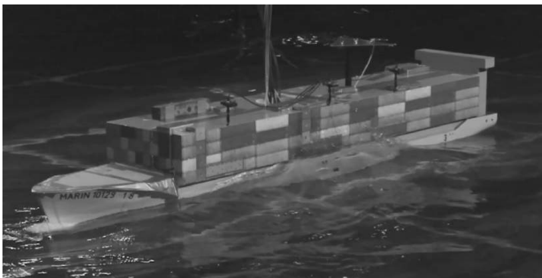
Figure 1-1: Green water loading on the lowest tiers of deck containers on a feeder ship, MARIN report 32558-2-OB
