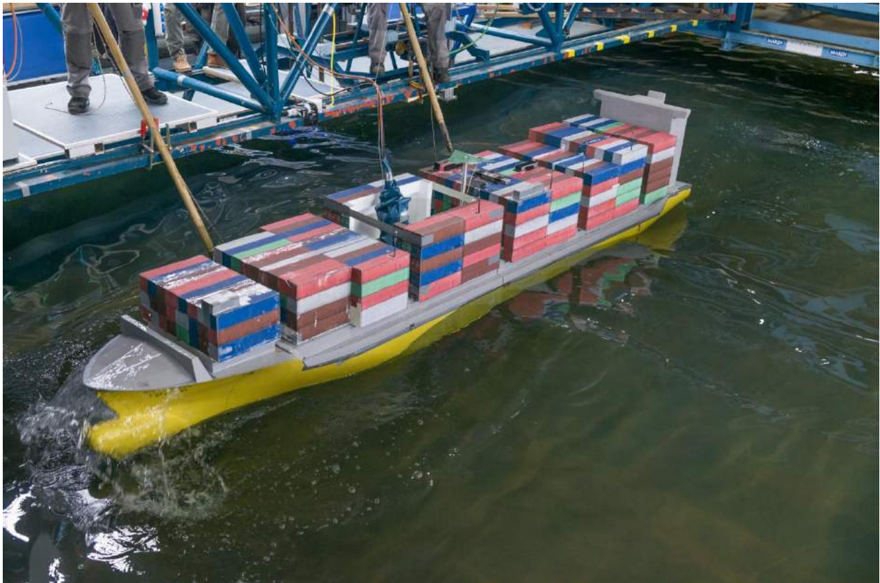
Photo 16 Test 33327_02BT_04_001: \mu = 180^\circ – H_s = 6.0 m – T_p = 11.8 s – V_s = 4 kn
