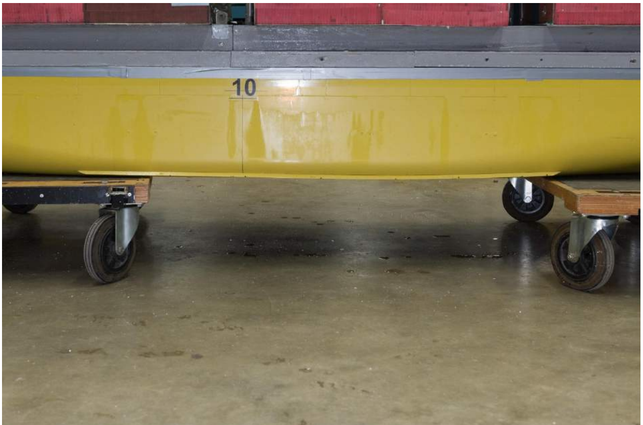
Photo 8 Details of the bilge keels – LC 2
