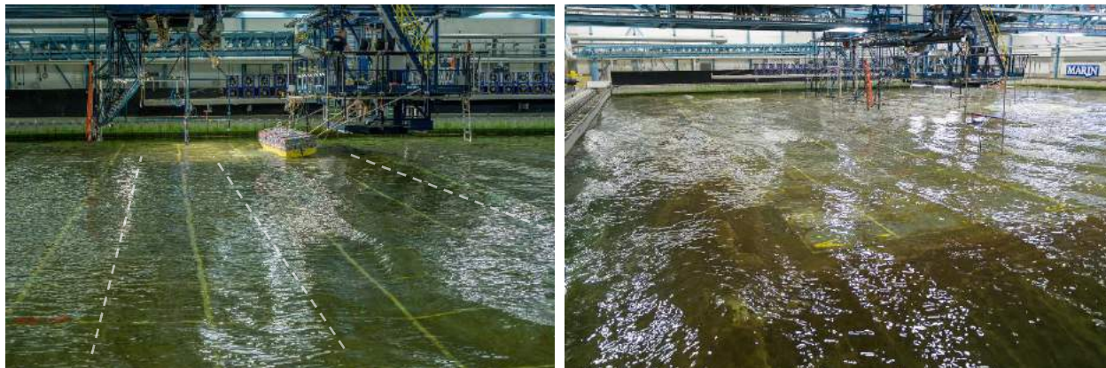
Figure 3-14: Long-crested waves (left) and short-crested waves (right). The dash lines underline the crest of the long-crested waves
