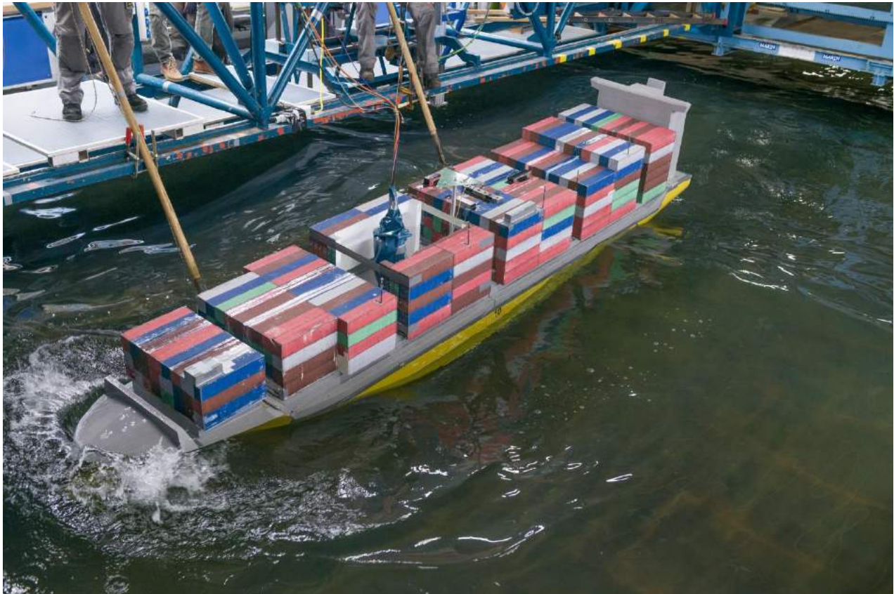
Photo 16 Test 33327_02BT_04_001: \mu = 180^\circ – H_s = 6.0 m – T_p = 11.8 s – V_s = 4 kn
