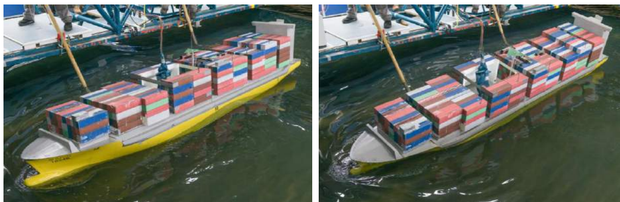
Figure 3-41: Occurrence of parametric roll during the test in head waves - Hs = 6 m, Tp = 11 s
