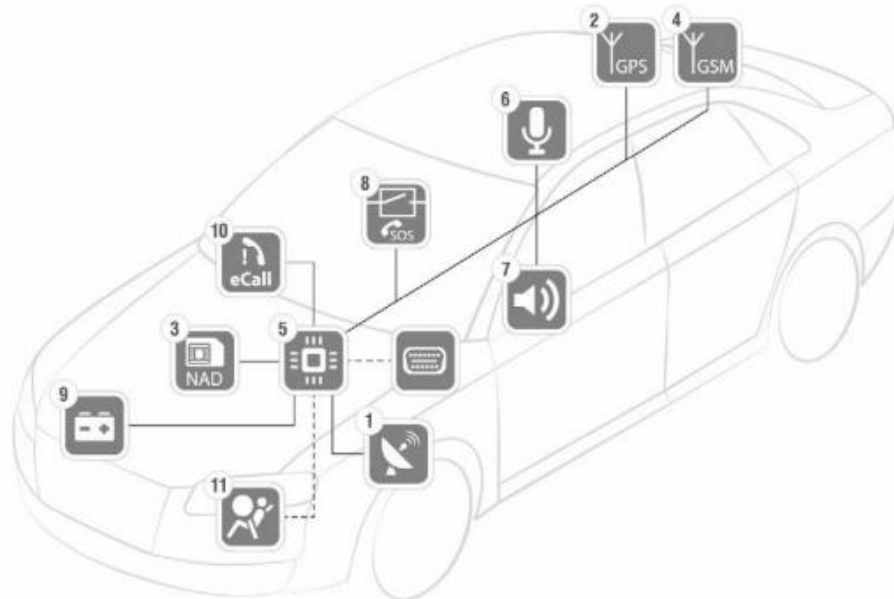
Figuur 2 eCall-boordsysteem, met verschillende functionele elementen [bron: Study on the inclusion of eCall in the periodic roadworthiness testing of motor vehicles, European Commission, January 2019 5 ]
