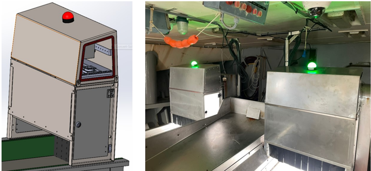
Figure 1. CatchWAM system. Concept (left) and two prototypes on board (right). Two systems are used because this vessel operated two conveyor belts to sort their catch.
